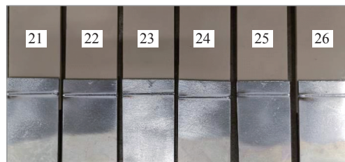
图4 铝合金(表面磷酸氧化)-聚醚醚酮激光连接试样 Fig.4 Laser direct joints of PEEK to Al (surface phosphoric acid oxidation)
